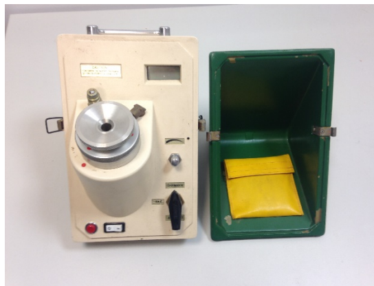
Fig. 5. Pressure chamber ARIMAD-2
