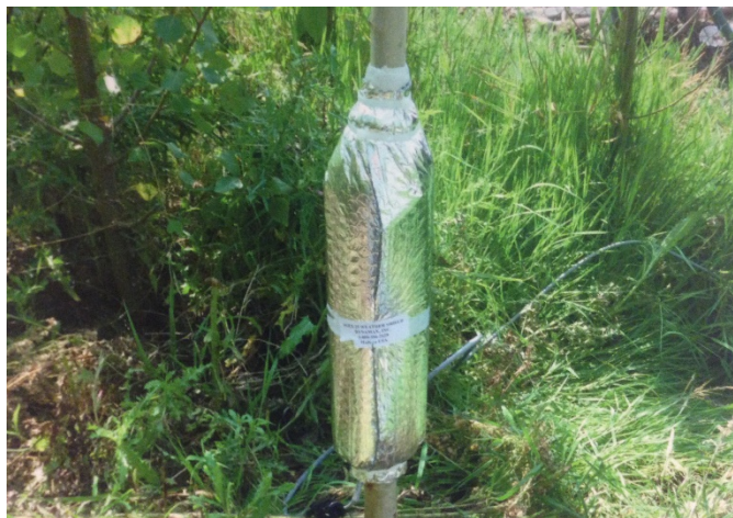
Fig. 3. Dynamax Sap flow meter mounted on a poplar stem.
