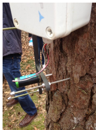
Figs. 6 and 7. Metal-belt and T-shape point dendrometer (resp. left and right)
