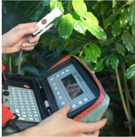
Fig. 4. Measurements of stomatal conductance with the AP4 porometer.
