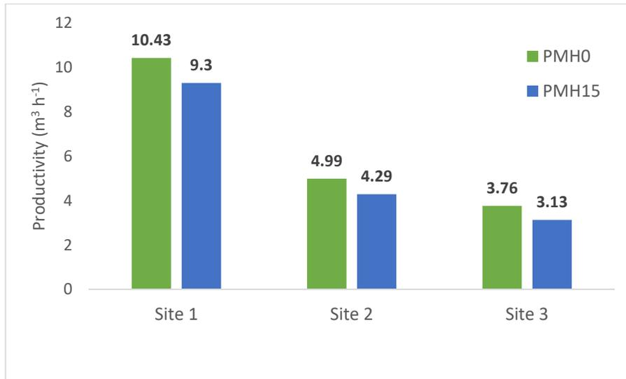
**Figure 11.** Net productivity (PMH<sub>0</sub>) and productivity including delays (PMH<sub>15</sub>)
