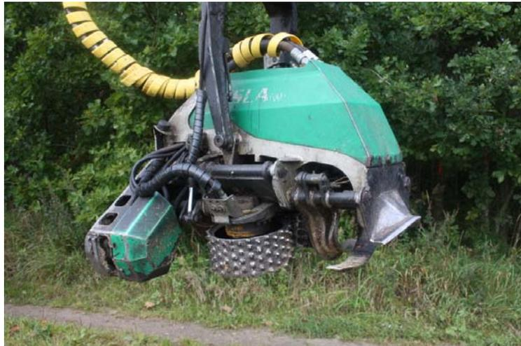
**Figure 9.** The Kesla head equipped to the harvester
