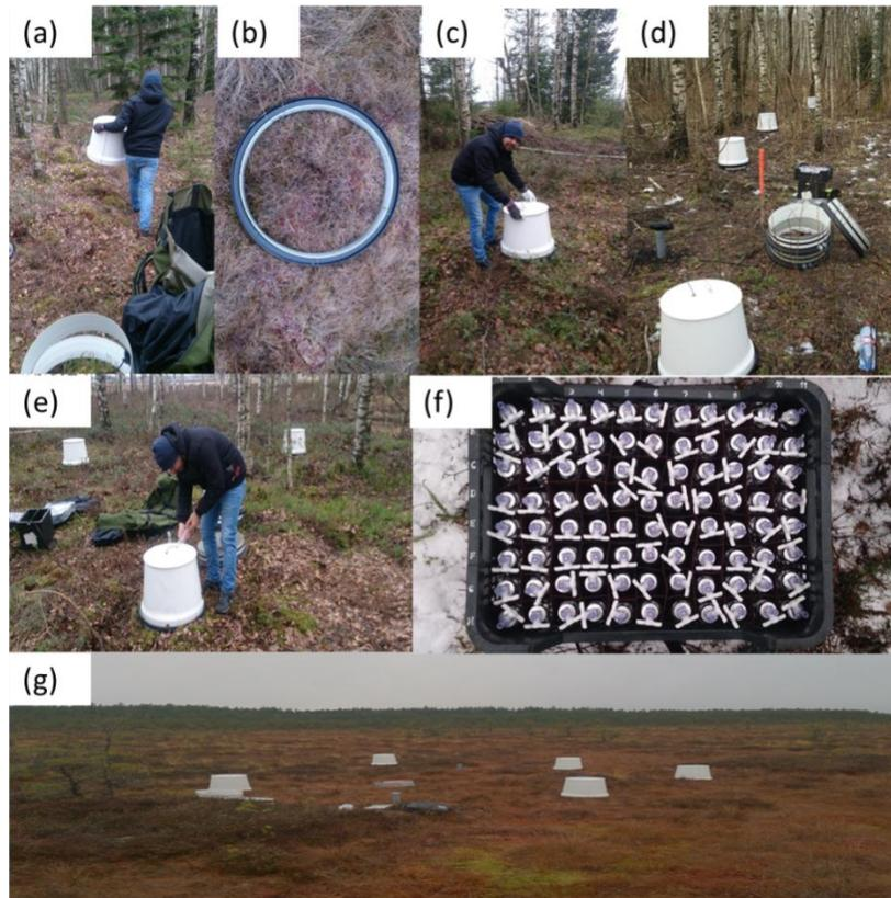
Figure 4. (a) carrying chamber (b) ring on the ground (c) covering ring by chamber (d) randomized sampling spots in natural forest on extracted peat lands (e) taking sample by using syringe (f) stored samples and (g) sampling spot on natural peat lands.
