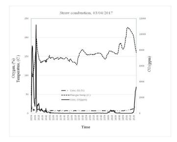
Fig. 3 - Evolution of straw combustion in 3 April trial concerning to the time variation of 3 variables.
