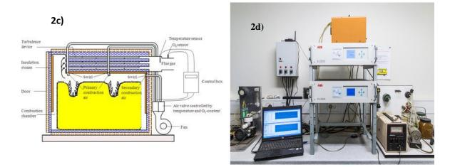
Fig. 2- Combustion equipment: 2a) feeding 500 Kg straw bale, 2b) burning, 2c) combustion chamber diagram and 2d) flue gas analysers.
