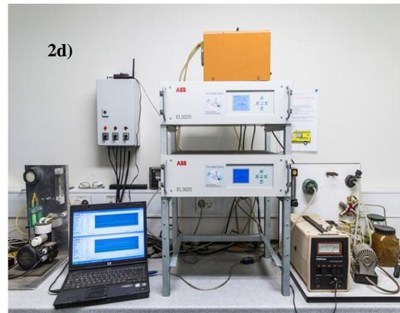
Fig. 2- Combustion equipment: 2a) feeding 500 Kg straw bale, 2b) burning, 2c) combustion chamber diagram and 2d) flue gas analysers.
