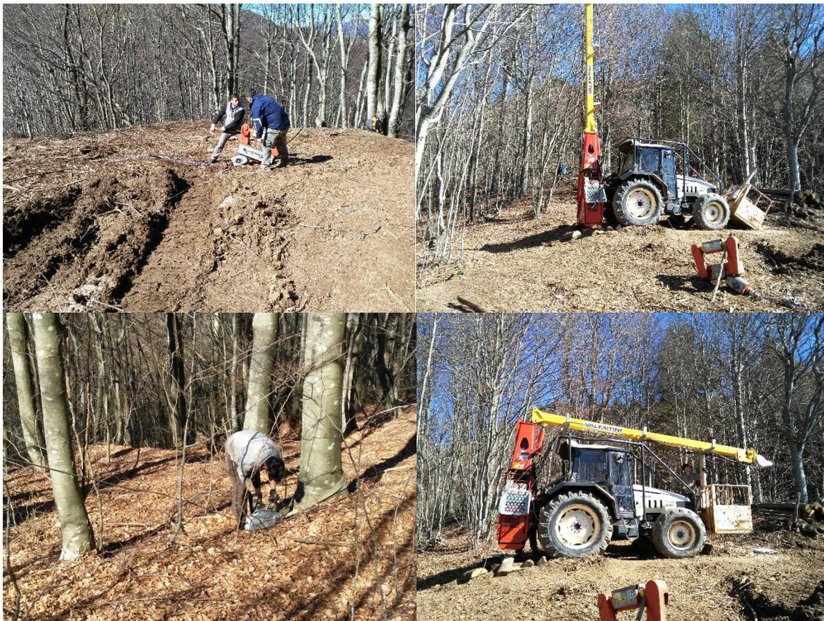
Figure 8: Disassembly of the equipment, up to the left downing the carriage, up to the right collecting the cables, down left removing anchorages and downright the equipment grouped.
