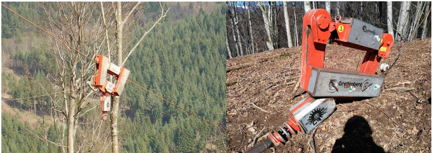
Figure 4 The carriages. Left Greifenberg CRG 25 (Picchi, G. 2017); Right Greifenberg CRG 15 (Navarro P. 2017)
