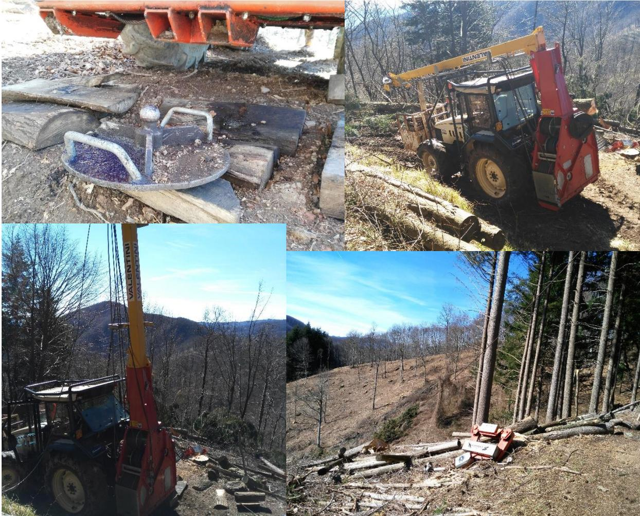
Figure 9 Up to the left the base of the tower (base plate), up to right position of the all equipment, down left mounting the tower, downright checking the main line and preparation of the carriage (Navarro, P. 2017).
