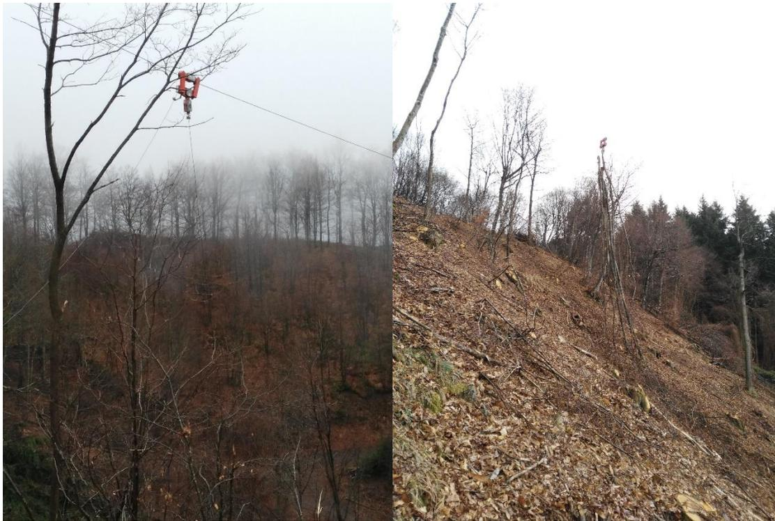
Figure 7 Left carriage downing the skidding cable and right carriage uploading the trees (Navarro, P., 2017)
