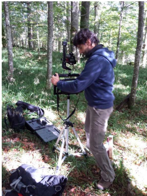
FIGURE 1 – Calibrating Field-Map compass before collecting data
