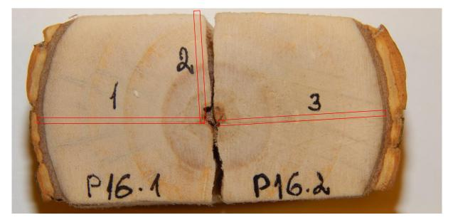
Fig.2. Sample P16 after LA-ICP-MS run (numbers 1, 2 and 3 indicate ablation patterns).
