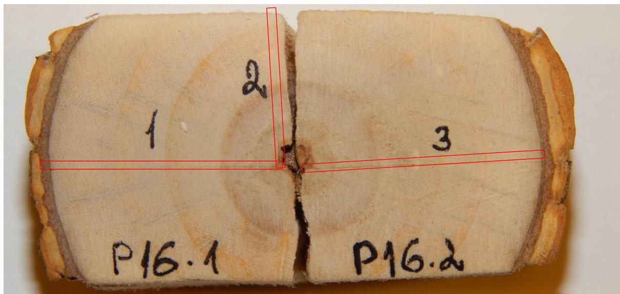
Fig.2. Sample P16 after LA-ICP-MS run (numbers 1, 2 and 3 indicate ablation patterns).
