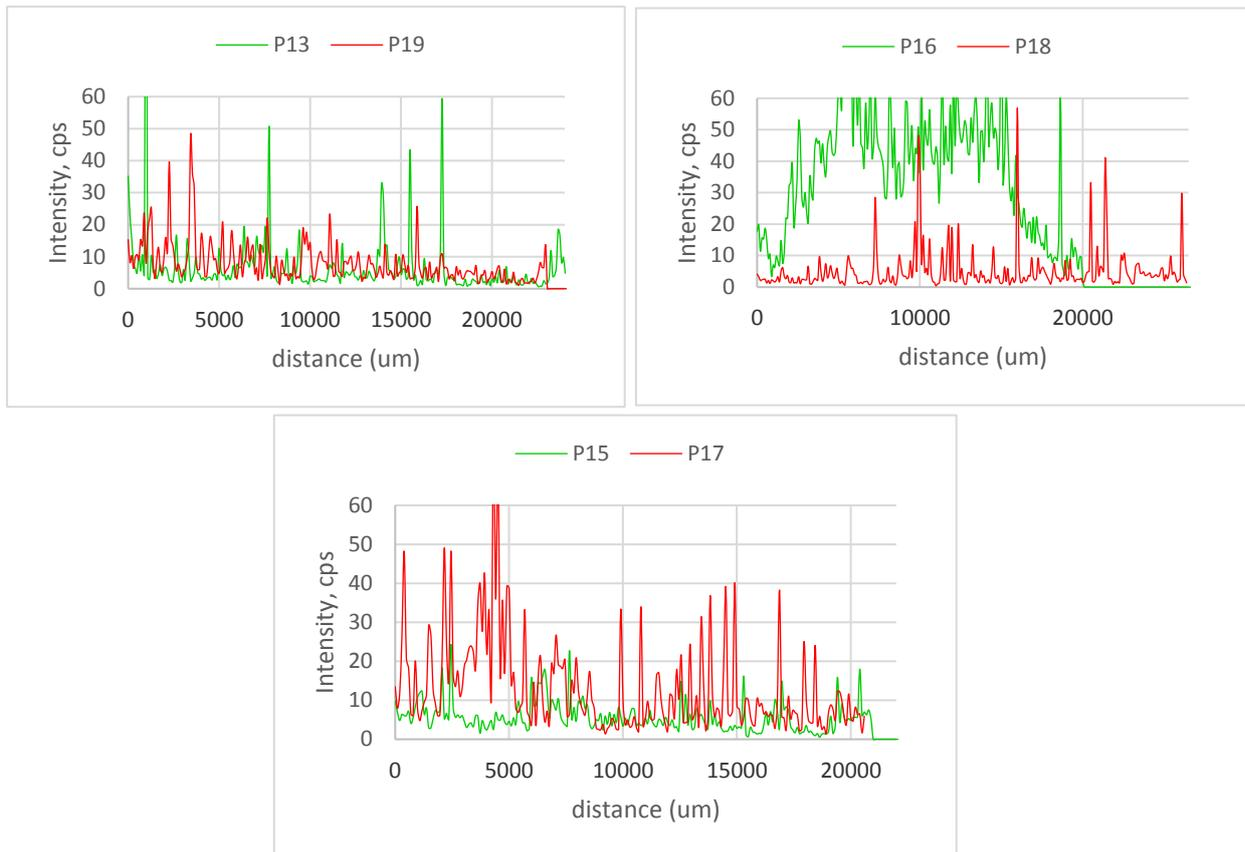
**Fig.7. Lead content in hybrid poplar clones AF2 (samples P13, P19), AF7 (samples P16, P18) and AF8 (samples P15, P17).**
