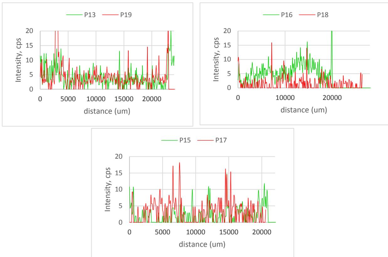
**Fig.6. Cadmium content in hybrid poplar clones AF2 (samples P13, P19), AF7 (samples P16, P18) and AF8 (samples P15, P17).**
