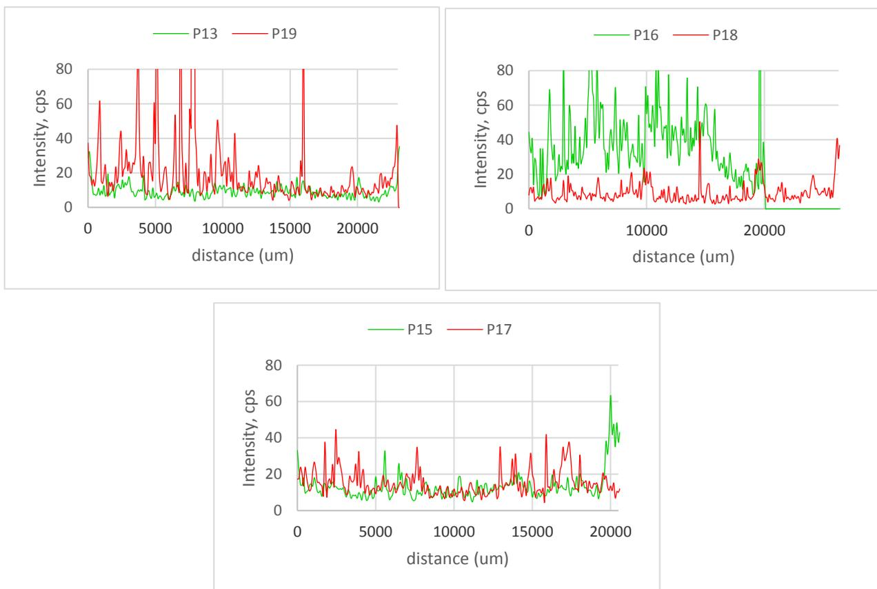
**Fig.5. Copper content in hybrid poplar clones AF2 (samples P13, P19), AF7 (samples P16, P18) and AF8 (samples P15, P17).**
