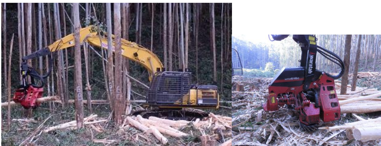
Figure 2 - Excavator Sumitomo equipped with Waratah head
