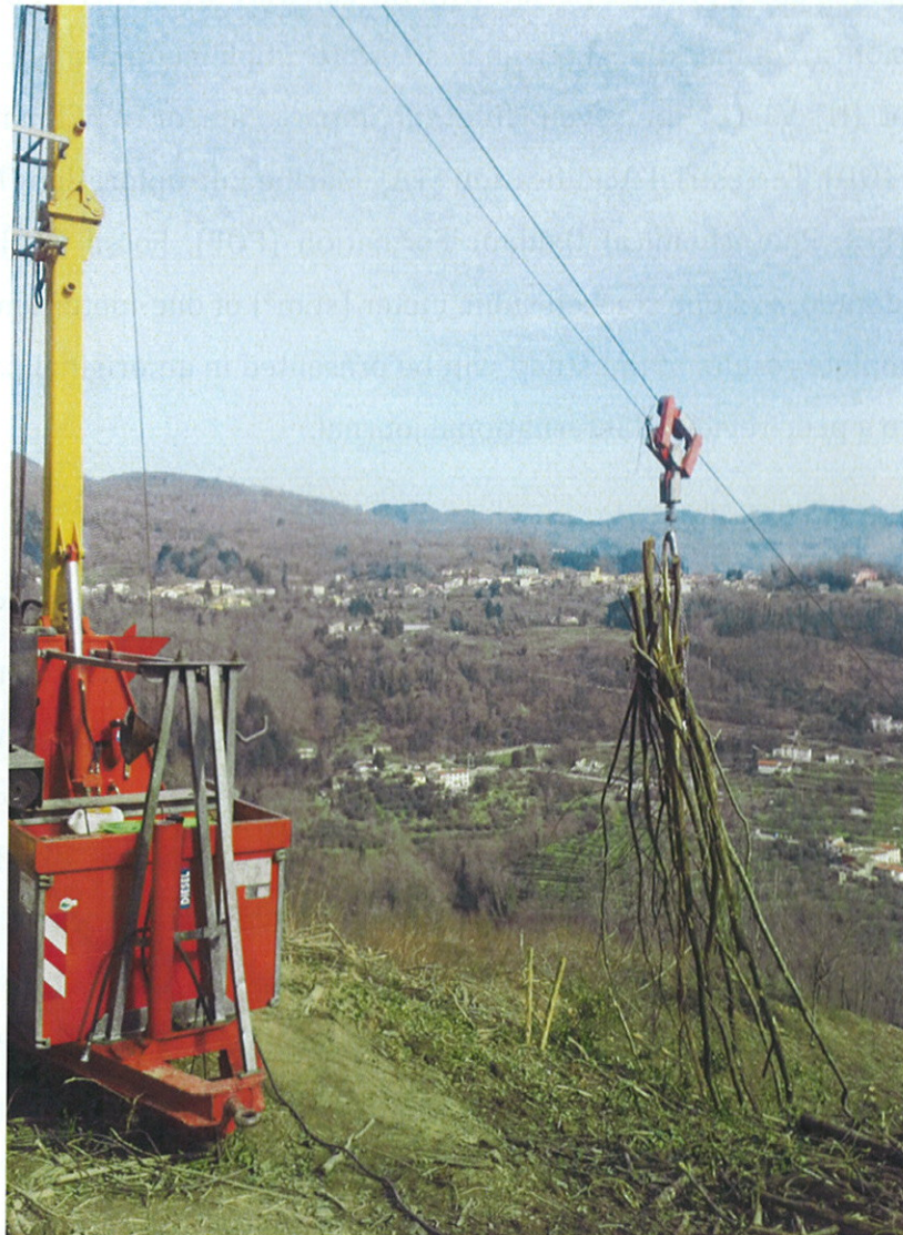
Figure 2. Extraction with cable yarder (Full Tree System).
