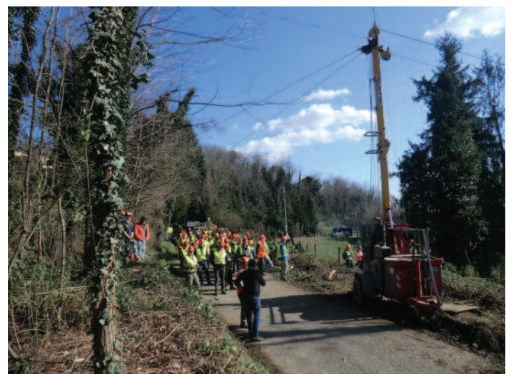
A 'cable yarding' system used to drag coppice poles up steep slopes in Italy.
