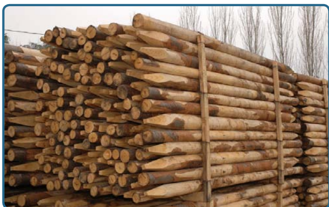
Figure 5. Chestnut poles that have been debarked and sharpened (Photo: Ivalsa)
