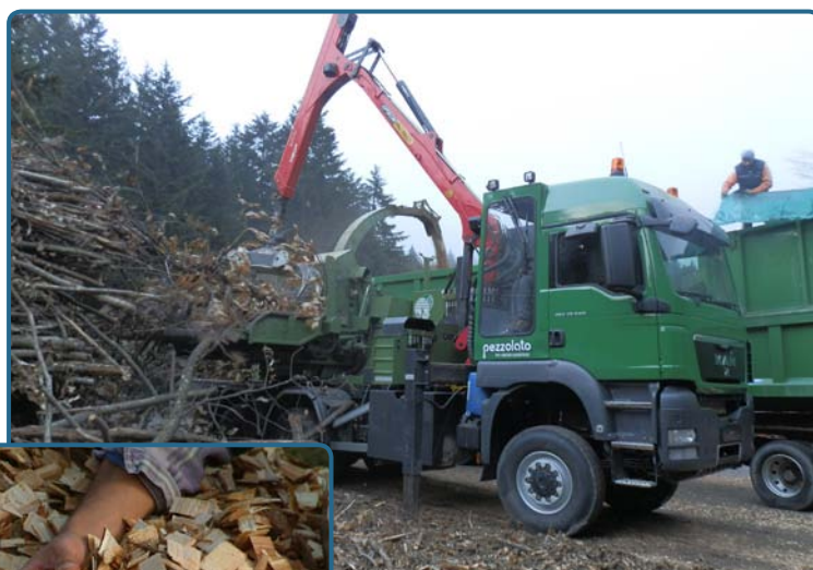
Figure 3. Chipper working at the landing, chipping coppice wood (Photos: Ivalsa)
