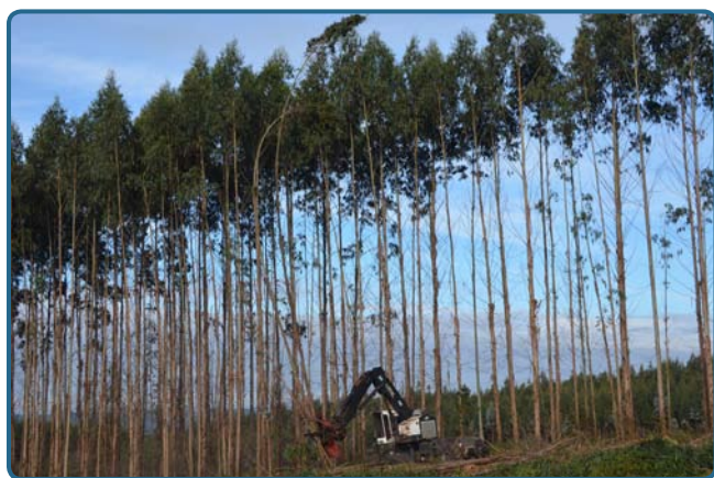
Figure 2. Mechanized felling and bunching in a eucalypt coppice (Photo: J. Carvalho)
