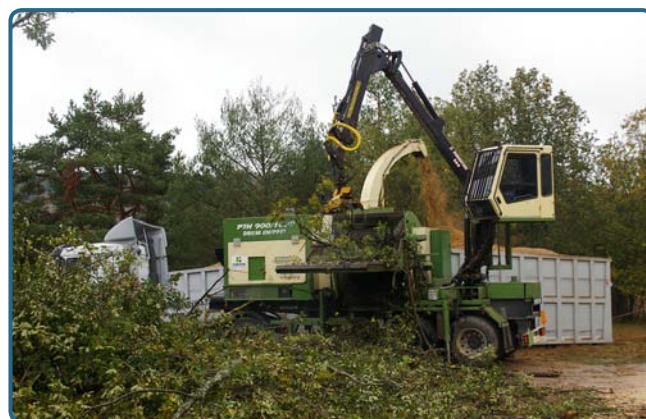
Figure 4. Coppice harvesting residues are chipped into renewable fuel (Photo: E. Tolosana)
