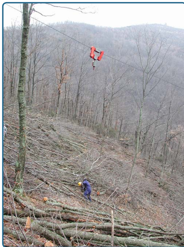
Figure 6. Cable yarder extraction is the best solution when site conditions are not favourable to machine access (Photo: R. Spinelli)
