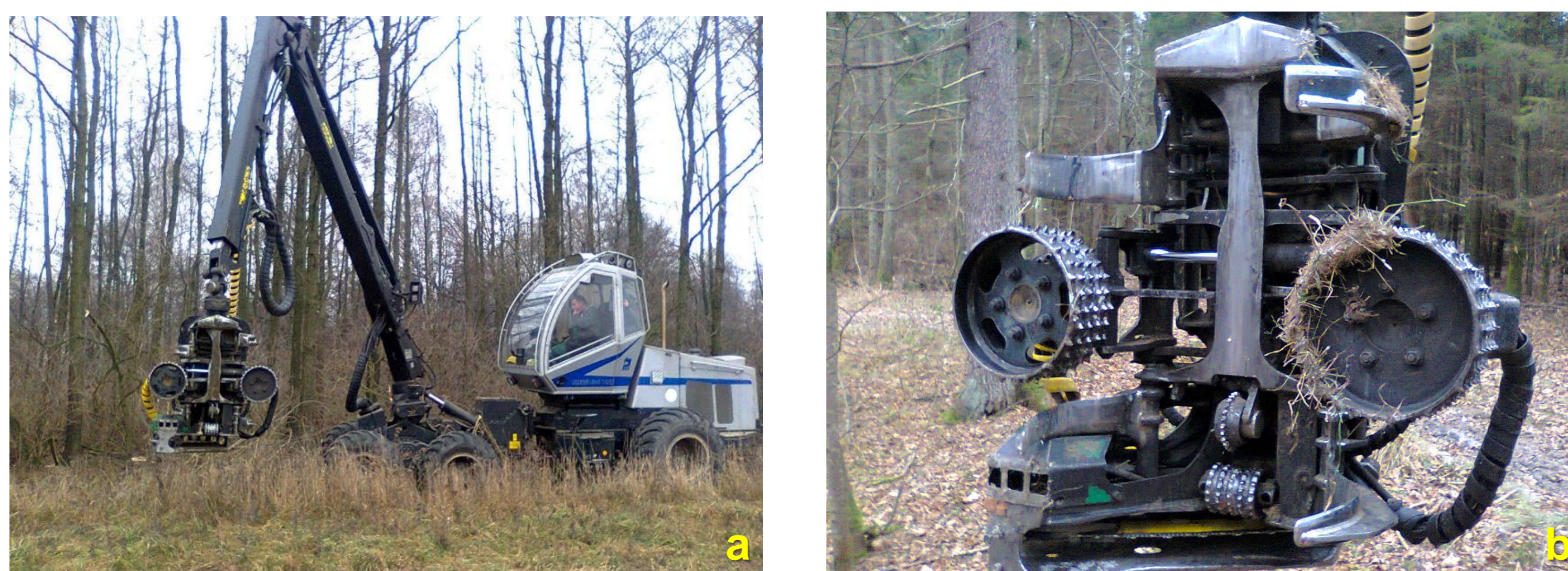
Figure 2. TBM 84V.II 6WD harvester (a), equipped with a Kesla 20 RH harvesting head (b)
