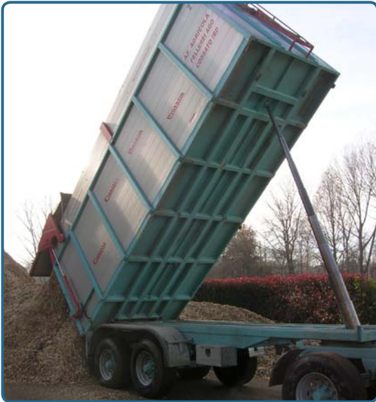
Figure 16. Unloading of chips; the chips should be used immediately if possible (Photo: J. Schweier)
