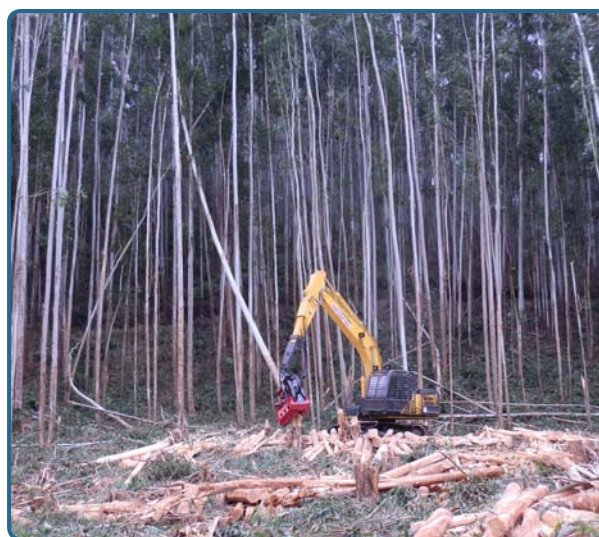
Figure 2. Mechanized industrial felling in a eucalypt SRF plantations managed as coppice (Photo 1 & 2: R. Spinelli)
