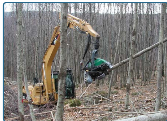
Figure 8. Mechanized cut-to-length harvesting (Photo: R. Spinelli)
