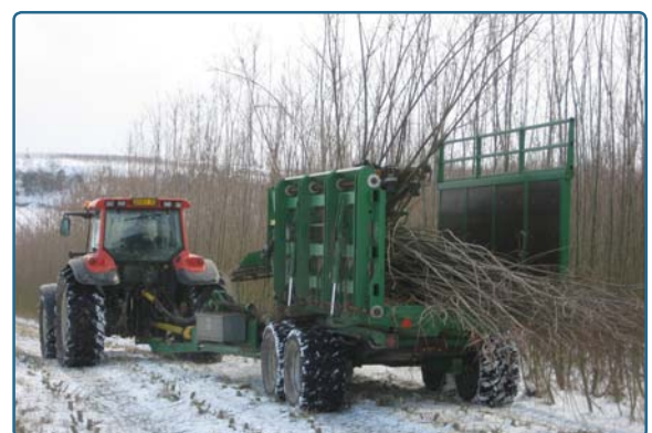
Figure 18. Example of the cutting in the double pass cut and store techniques. The stems will be chipped later (Photo: J. Schweier)
