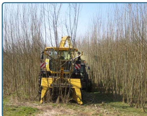
Figure 3. Single-pass harvesting in SRC established with willow (Photo: J. Schweier)
