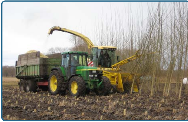
Figure 17. Examples of single pass cut-and-chip system: the harvesting machine cuts and chips the stems and the chips are discharged directly into a tractor-trailer units. (Photos: J. Schweier)
