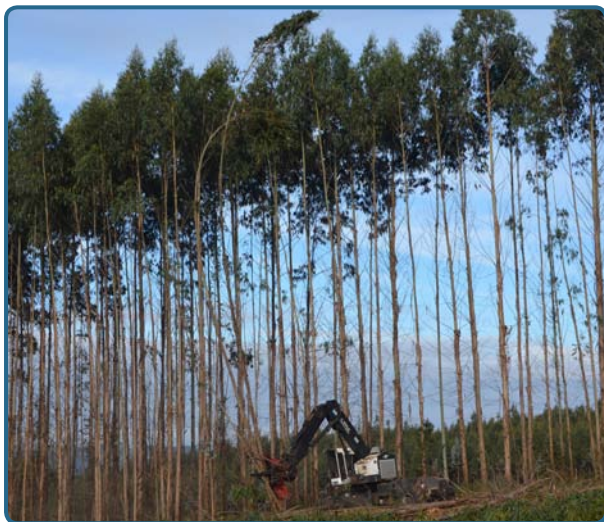
Figure 2. Mechanized felling and bunching in a eucalypt coppice (Photo: E. Tolosana)
