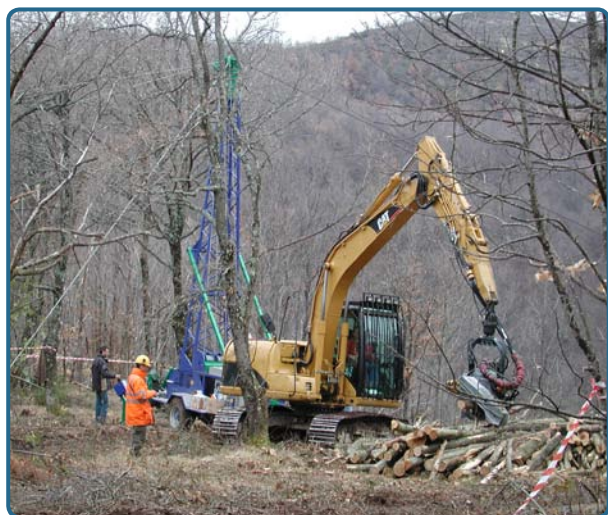
Figure 5. Processor and yarder (Photo: R. Spinelli)
