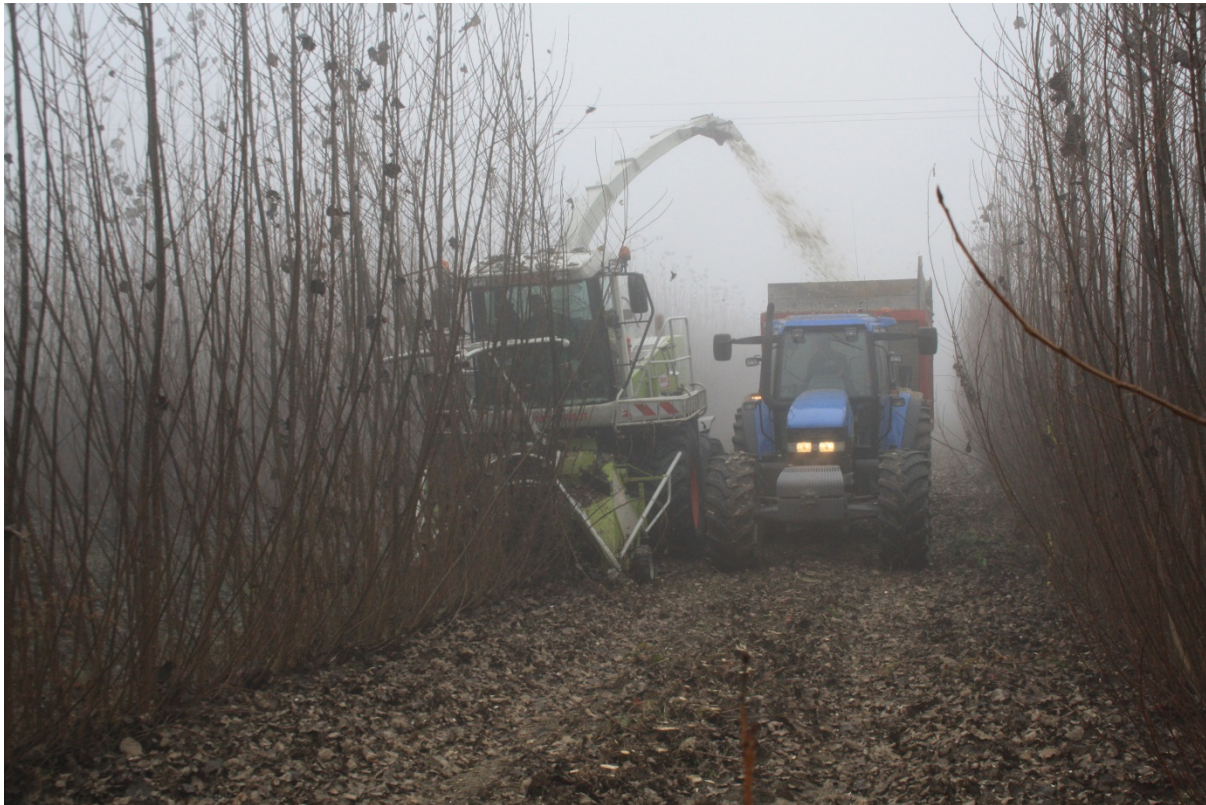
Figure 2. The Veneta Mais coppice header at work in a single stem, two year old short-rotation coppice in Musile di Piave (Italy).
