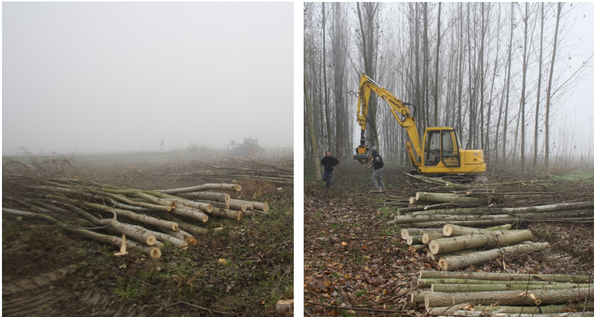
Figure 3. Harvesting trial at Allasia with the GMT035 forest harvester. Left: stems harvested for complete chipping. Right: stems harvested partially for logs and partially for chipping
