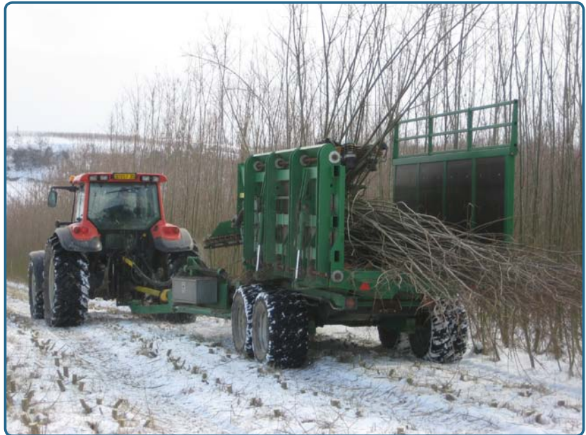
Figure 18. Example of the cutting in the double pass cut and store techniques. The stems will be chipped later (photo: J. Schweier)
