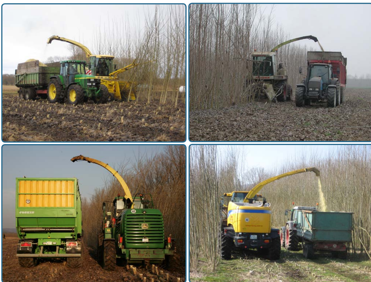
Figure 17. Examples of single pass cut -and-chip system: the harvesting machine cuts and chipped the stems and the chips are discharged directly into a tractor-trailer units. (photos: upper-right R. Spinelli, rest J. Schweier)
