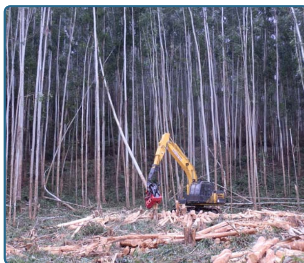
Figure 2. Mechanized industrial felling in a eucalyptus SRF plantations managed as coppice (photo 1 & 2 R. Spinelli)
