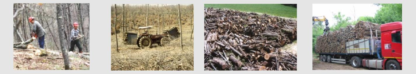
After extraction firewood is manually loaded onto trucks by two or three operators standing on the truck while a loader lifts the firewood to be stacked. This work phase is one of the most dangerous of the whole process and the risk to slip or to fall is very high.
