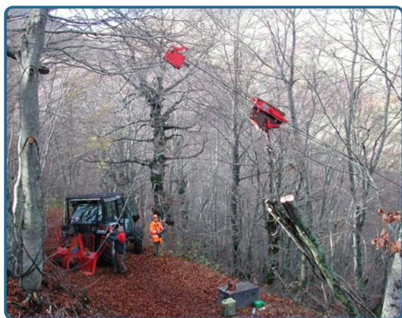
Figure 9. Cable yarding on steep terrain (Photo: R. Spinelli)
