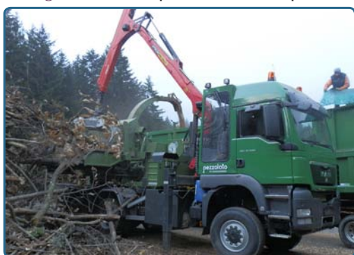
Figure 3. Chipper working at the landing, chipping coppice wood
